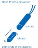
Both ends of the magne work equally well
