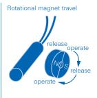
Multi-pole ring magnets can be used to achieve a larger number of operations per rotation
