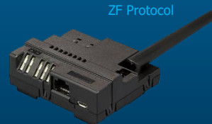
Packaged RF Receiver AFZE-1003, 868 MHz AFZE-5003, 915 MHz
