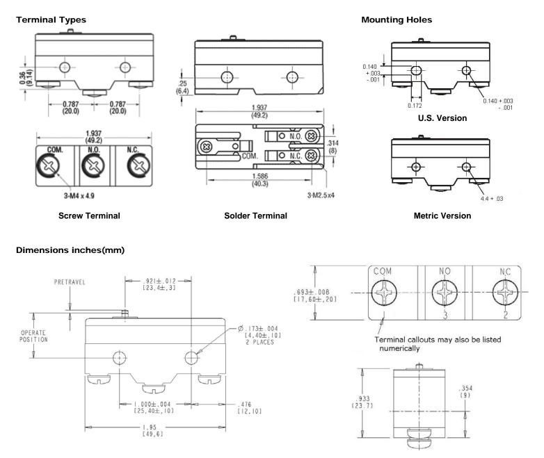
Note: GP Series switches are available with screw or solder terminals and with U.S. or metric holes
