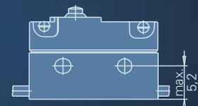
Model with leads, 5,2 mm from base to drill hole
