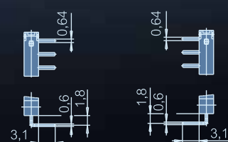
PCB terminal RH-side
